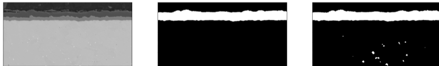
Figure 10: SEM Image, Ground Truth, and Model Prediction with \text{IoU} \approx 87\%
